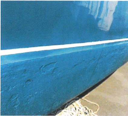
Photo above: Rough antifoul surface damages hull performance
